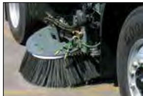
In-cab side broom tilt and extended reach
