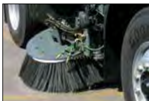
In-cab side broom tilt and extended reach
